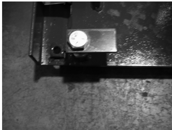
Figure 9d - Proxy sensing plate locate at the front of the baseframe
